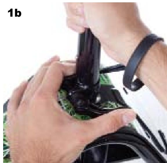
2. Remove the two bolts holding the top cap onto the steering mast. Lay the handlebar on the steering mast, then replace the top cap and tighten the two bolts securely and evenly (7Nm (62 in-lbs)). If you need to rotate the handlebar to move the brakes and throttle to a more comfortable position, simply loosen the two bolts then re-tighten when done.
