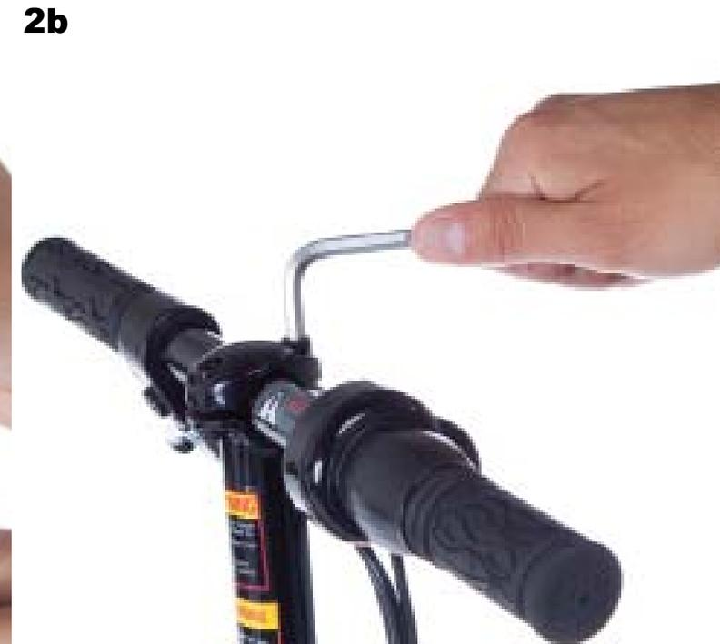
3. Before riding for the first time, you should check the tightness of all nuts and bolts on the scooter. Most important are the front wheel axle nuts, any nuts or bolts around the rear brake, the motor, and the rear wheel. Make sure the brake levers and throttle are secure on the handlebars; if they can be twisted out of alignment, their mounting bolts need to be tightened.
