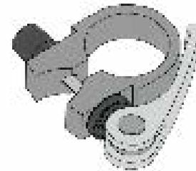
5. If you are able to force the handlebar out of alignment with the front wheels, the clamp needs to be adjusted. Holding the quick release lever in the OPEN position with one hand, tighten the tension adjusting nut with your other hand about 1/2 turn clockwise.
