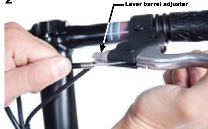
*Cable is drawn through brake lever. Note the gap in the barrel adjuster that allows the cable to pass through.*
