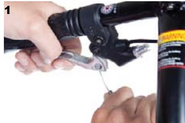
*Cable end fits into brake lever body*
